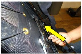
STEP 10: MOVE ADJUSTERS TO THE FORWARD POSITION AND TIGHTEN REAR NUTS THEN MOVE ADJUSTERS TO THE REAR POSITION AND TIGHTEN FRONT NUTS.
