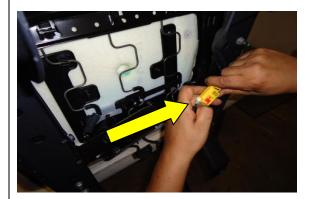
STEP 3: DISCONNECT ALL OTHER CABLES UNDER THE SEAT. (SEAT HEATER, AIR BAG, SEAT BELT SENSOR)
