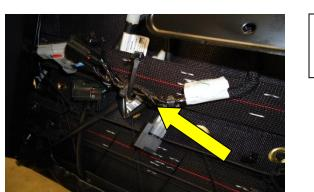
STEP 11: CONNECT THE SEAT BELT SENSOR DEVICE TO THE CABLES AND USING ZIP TIES ATTACH THE LOOSE CABLES TO THE SEAT.
