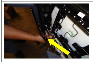
STEP 5: MOVE ADJUSTERS TO THE FORWARD POSITION AND UNBOLT THE (4) REAR ADJUSTER NUTS. RETAIN THE NUTS FOR LATER USE.
