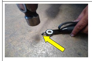
STEP 9: BEFORE ATTACHING SEAT BELT RECIEVER TO THE INBOARD SIDE OF THE SEAT, TAB MUST BE BENT FLAT.
