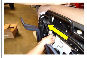
STEP 4: MOVE ADJUSTERS TO THE REAR POSITION AND UNBOLT THE (4) FRONT ADJUSTER NUTS. RETAIN THE NUTS FOR LATER USE.
