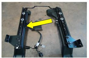
STEP 6: REMOVE FACTORY ADJUSTERS FROM FACTORY SEAT AND PLACE TO THE SIDE. DISCONNECT REMAINING SENSOR FROM THE ADJUSTERS AND RETAIN FOR LATER USE.
