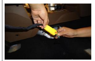
STEP 12: PLACE SEAT IN VEHICLE AND LINE UP MOUNTING HOLES TO MOUNTS AND CONNECT THE SENSOR CABLES.
